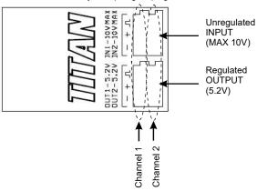
**Warning:** Under heavy continuous current load, the Titan unit will get extremely hot and cause burns when touched. Allow unit to cool before handling.
